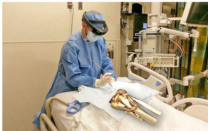
Figure 1.5.: Interpretation of operating room scenario: surgeon with AR Head-Mounted Display sees rendering of segmented CT data while operating [38, 88]
