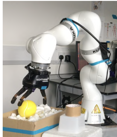
(b) Hand mounted on robot arm (source Koenig et al. [39]).
