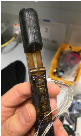
Figure 2.4: Barometric pressure sensors integrated in the robotic fingers.
